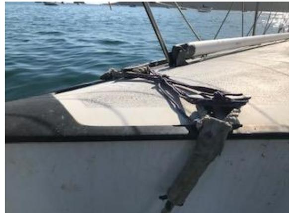
Here, firehose is used at the edge of the deck to protect the bridle lines. It can be challenging to keep the fire hose in the correct spot. By making a hole in the fire hose in the correct spot then using zip ties or twine to wrap the bottom of the eye keeps chaffing "gear" in the correct position. If possible check thimbles for chaffing or damage where the line connects to chain contact Harbor Patrol or the Mooring Crew if you notice any damage.
