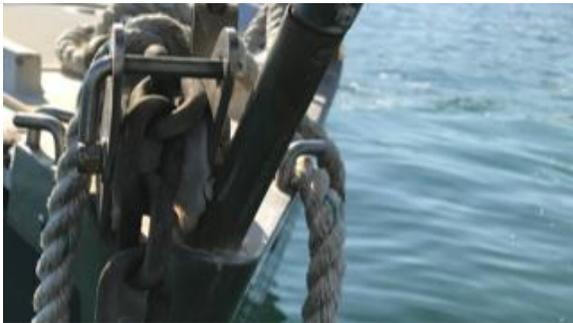
If a chain is chaffing on wood or fiberglass during a storm it will start to saw through the vessel causing damage. If your chain has a hook on it insure the clasp spring is operational or find another way to secure.
